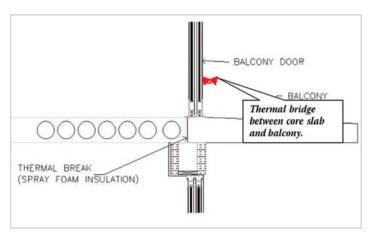
Figure 6 Construction detail showing thermal bridging at wall-balcony interesection
