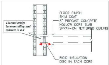
Figure 5 Thermal bridge at wall-floor slab intersection
