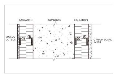
Figure 2 Wall cross-section schematic showing sensor locations
